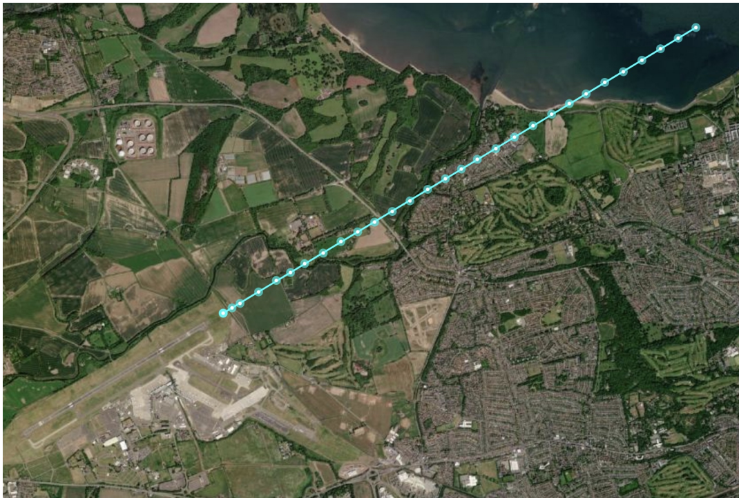
Figure 3.5: ADS-B message locations for airplane on short final for Edinburgh Airport runway 24 (satellite image © 2023 Esri)
